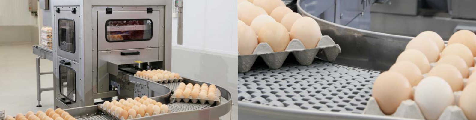
Automatic destacking of transport trays
